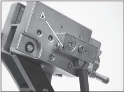
Loosen the 1.5 mm locking set screw (A) located on the side of the latching block as shown. The set screw is used to hold the adjustment screw in place.
