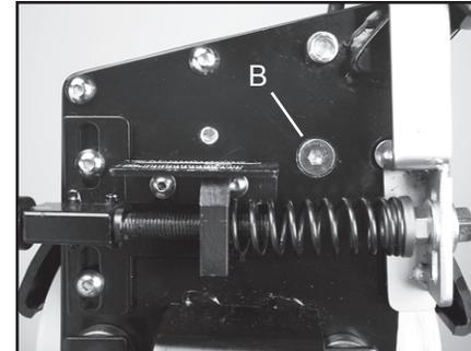
While holding the 5mm brake lever adjustment bolt (A), loosen the hex bolt (B) located on the back side of the tensioner frame with the 4 mm allen wrench.
