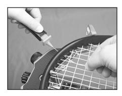
Once the awl is inserted, pull the handle of the awl outward while holding the tip section in place. This leaves the outer sheath in the grommet hole. Insert the end of the string into the outer sheath.
