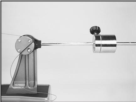
When the correct tension is attained, the drop weight bar will rest horizontally as shown. For accurate tensioning, it must be lowered and come to rest at horizontal without assistance. Manually forcing the tension bar to the horizontal position will greatly increase the string tension and may result in racquet damage. If the tension bar comes to rest above horizontal, release the string by lifting the bar and re-pull the string.
