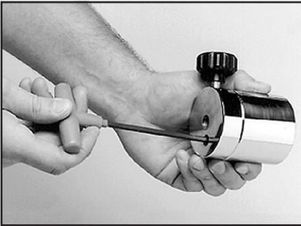
The drop weight is of a two piece design. When assembled, it will accommodate tensions from 20 to 90 lbs. For tensions from 8 to 20 lbs., remove the 5mm bolt on the face of the drop weight, and use the smaller portion of the weight as described above.
