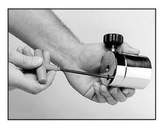
The drop weight is of a two piece design. When assembled, it will accommodate tensions from 20 to 90 lbs. For tensions from 8 to 20 lbs., remove the 5mm bolt on the face of the drop weight, and use the smaller portion of the weight as described above.
