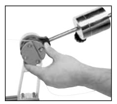
While holding the string gripper drum with your hand, lift the tension bar to approximately 45 degree angle and let fall. If the tension bar drops below horizontal, repeat the above action until the bar comes to rest parallel to the racquet. The set tension will be reached when the bar rests horizontal.
